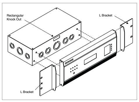
Figure 1-3 L Brackets for Rack Mounting
